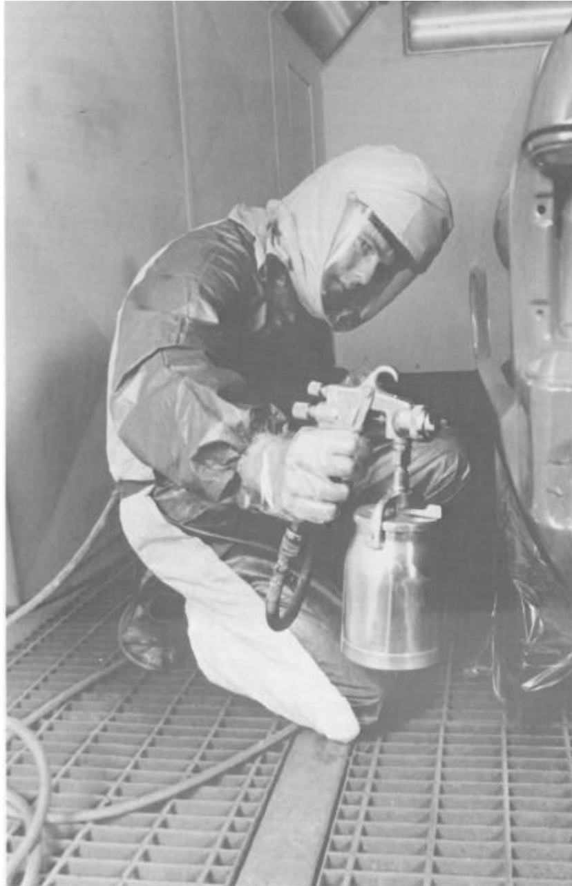
Using personal protective equipment to spray isocyanate - containing paint
